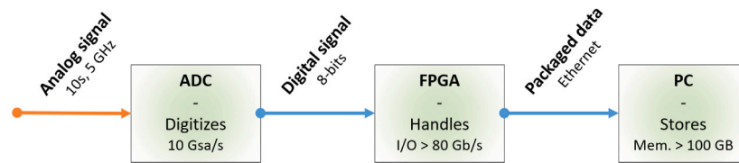
Fig. 1. Schematic overview of the acquisition system and requirements established in Section 2: an analog signal (left) of specific duration and bandwidth arrives at the device. It is digitized by the ADC at the required Nyquist rate. The FPGA then handles the digital data faster than it is received and sends it to storage on the PC's memory. These requirements avoid memory overflow on any shown component.
