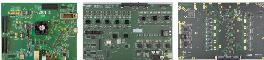
Fig. 1 Full-stack ECHo DAQ SDR electronics: digital processing board (left); analog/digital conversion board (center); high-frequency analog heterodyne mixer board (right)
