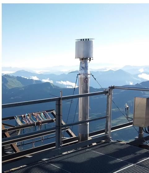
Figure 5.3.: Aerosol inlet on the rooftop of the SBO station.
