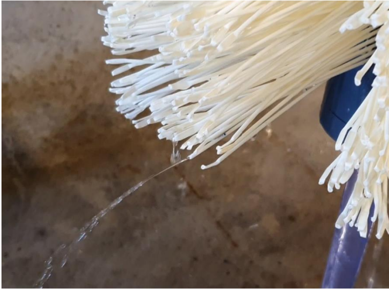
Figure 6.3. Leakage identification on HF membrane module
