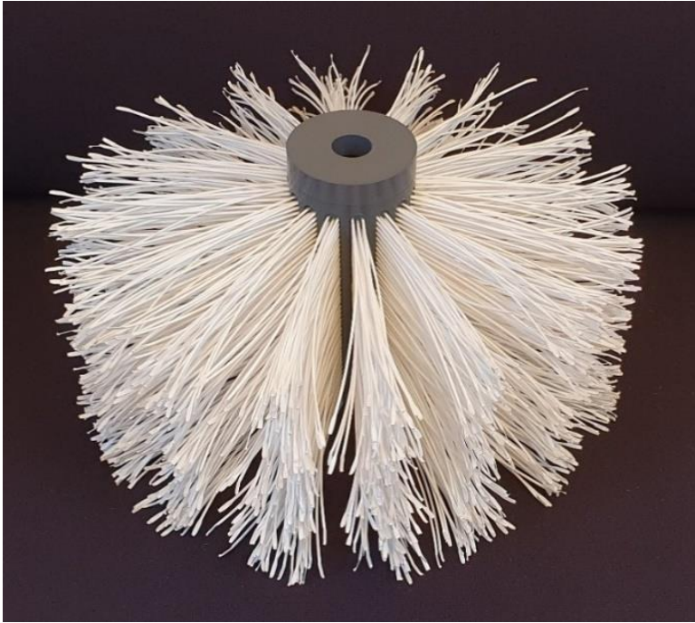
Figure 3.1. Rotatable membrane prototype system with 1,950 horizontally aligned hollow fibres
