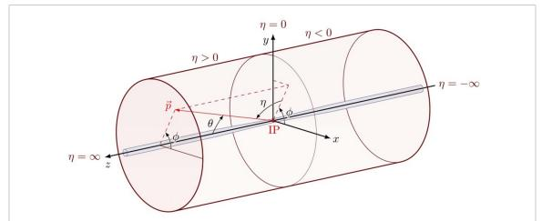
**Figure 1.** The CMS coordinate system, which explains the particle's motion within the cylindrical detector. Figure adapted from https://tikz.net/axis3d\_cms/.
