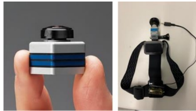
Fig. 2. Micro HDR imager, aka. the “VIP” camera. This camera was equipped with a fish eye lens and a head strap to be used as a wearable [16].
