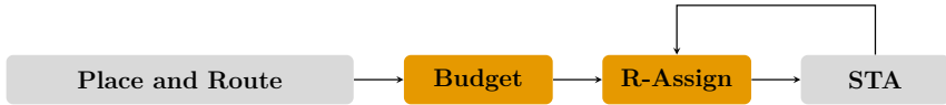
Figure 7.5: VPR extensions to support mapping applications to regions with dynamically assigned modes. The Budget slack estimation pass and the R-Assign mode assignment pass shown in orange have been newly added to the original VPR flow.
