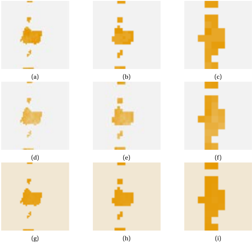
Figure 10.24: Aging compensation for the arm_core benchmark, evaluated using the RFET model and t = 10y . Rows show from top to bottom: Achieved delay, control voltage and relative power. Columns show different regions sizes. From left to right: 5x5, 10x10 and 25x25.
