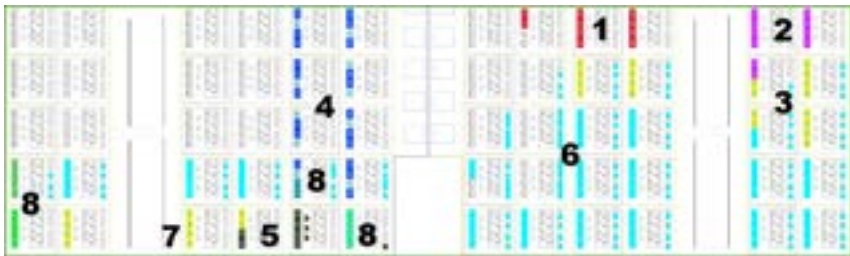
Figure 9.4: VFPGA tile (type 9) placed using the manual placement strategy. Multiplexers of the PSM’s top, right, bottom and left side are marked red (1), purple (2), yellow (3) and blue (4). The CLB is located at the bottom with the LUT, two internal multiplexers and D-flip-flop colored in black (5). Sky blue color represents the configuration units of the tile (6). Yellow blocks at the bottom (7) depict Write Connection Boxes, whereas Read Connection Boxes are marked green and turquoise (8) and make up remaining logic distributed around the LUT.
