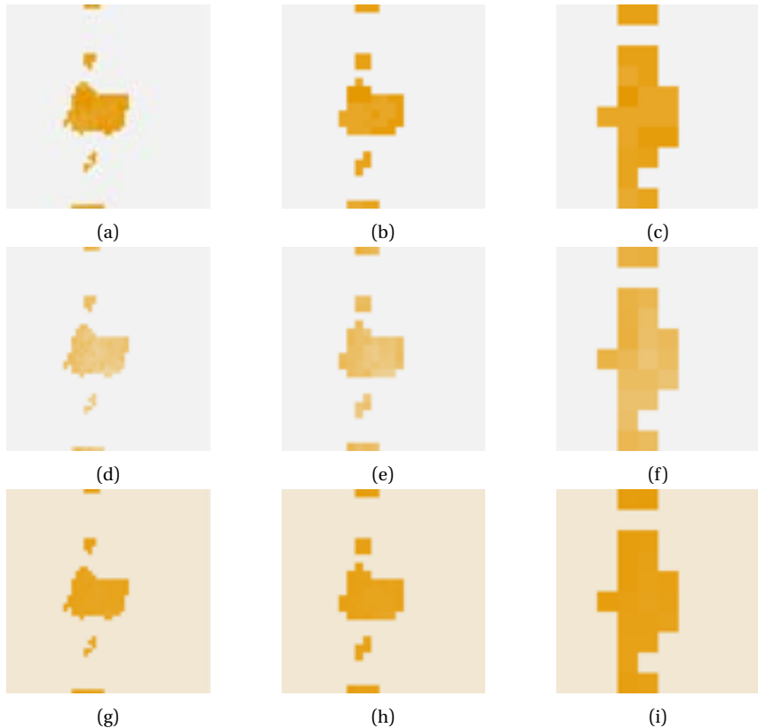
Figure 10.21: Temperature variation compensation for the arm_core benchmark, evaluated using the RFET model and T = 100 . Rows show from top to bottom: Achieved delay, control voltage and relative power. Columns show different regions sizes. From left to right: 5x5, 10x10 and 25x25.
