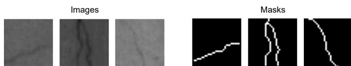
Figure 2: Sample images of cracks with corresponding masks.
