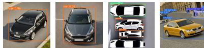
Figure 5: Bounding Boxes detected with YOLOv8x. This allows to crop the image and provides a confidence score for the presence of a car. It also allows to automatically sort out the two undesired images on the right where more than one car is detected.
