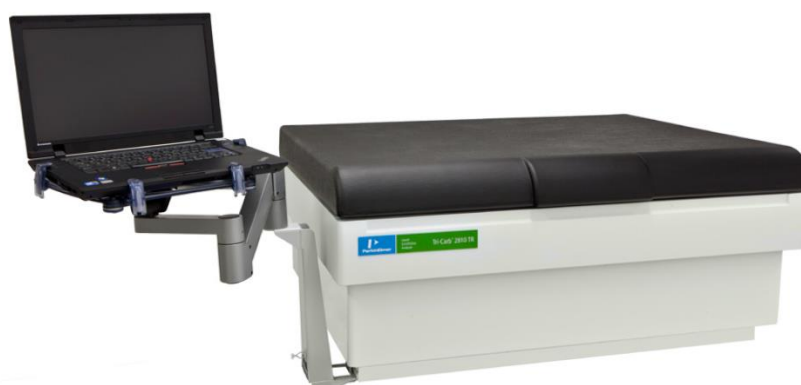
Figure 21: The LSC device Tri-Carb 3110 TR from the company PerkinElmer for measurements of \alpha or \beta emitters.
