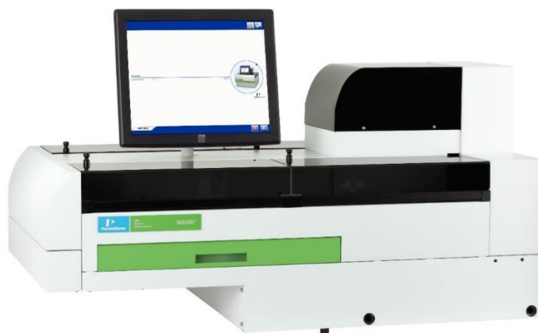
Figure 20: The \gamma -counter device, including a thallium doped single NaI crystal to measure Eu-152 samples among others.
