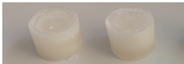
Figure 1 Pictures of ss-PCMs synthesized with Crodatherm 21.
