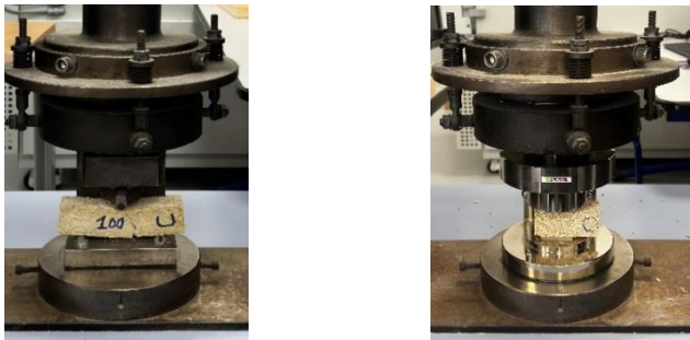
Figure 4 : experimental apparatus for bending (left) and compression (right) tests
