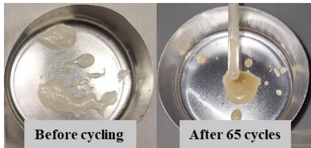
Figure 6: Change of color of Erythritol before cycling and after 65 cycles
