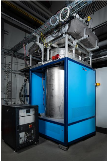
Figure 1: 400kg nitrate molten salt test rig for component testing at DLR
