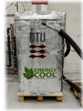
P2: 230 l salt hydrate (304 kg)
