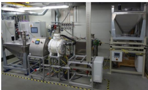
Figure 1: Laboratory Prototype of Thermochemical Long-Term Storage based on Quick Lime and Water
