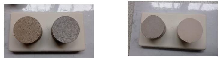
Figure 2. Pictures of 50 mm pellets scaling up manufacturing process; right CPCM1 and left CPCM2.
