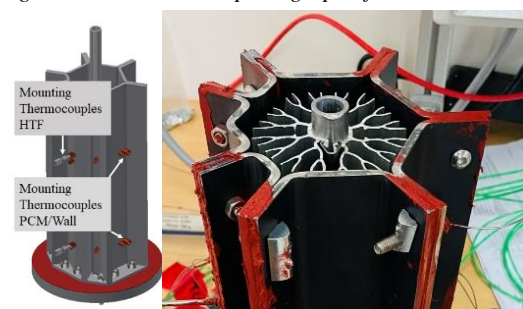
Figure 4: Schematic and photograph of the test container.
