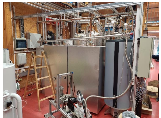
Figure 2: Real demonstrator in the laboratory at AEE INTEC (high temperature Storage to the right followed by sorption storage S1 and S2 and condenser/evaporator to the left and the heat pump behind the C/E
