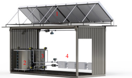
Figure 3: System concept 1) Solar collector, 2) Hot TES tank, 3) Cold TES tank, 4) Fan coils
