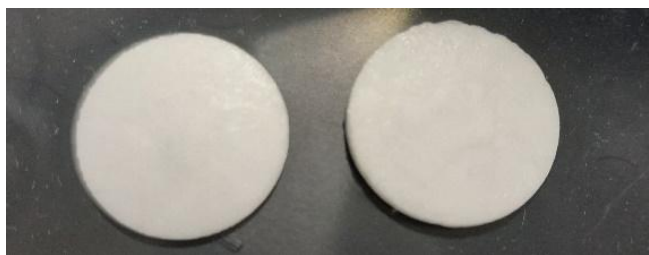
Figure 1: Samples obtained by pressing (left) and casting (right).
