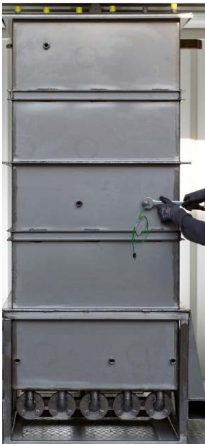
Figure 1: Side view of PCM-TES module before thermal insulation, showing threaded fittings for thermo-couple integration
