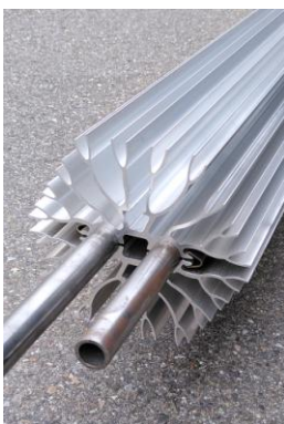
Figure 2 Dual-tube assembly consisting of steel tubes and aluminum fins.
