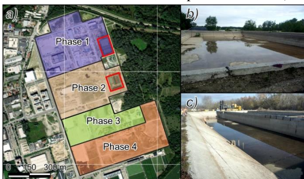
Figure 1: Construction phases at the IN-Campus (a; available basins highlighted in red), and pictures of the available basin structures (b: basin A, c: basin D). Aerial image: LDBV (2023).
