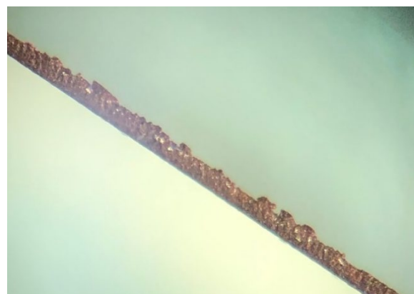
Figure 6. Optical image with a view on the side of the tape used for winding PC1. Large precipitates can be seen on the tape surface, leading to a strong increase of the effective conductor thickness in the winding.
