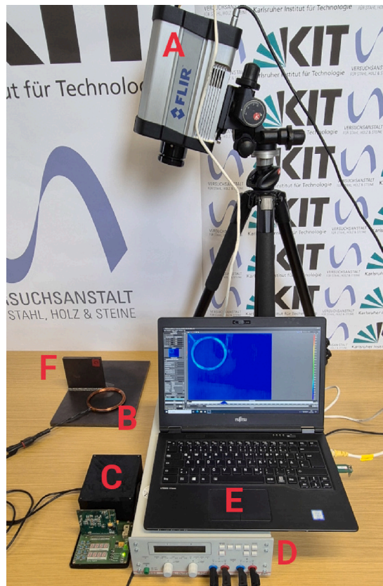
Fig. 4. Alternative crack detection setup. A: IR camera, B: coil, C: S2S unit, D: voltage supply, E: PC and F: steel specimen.
