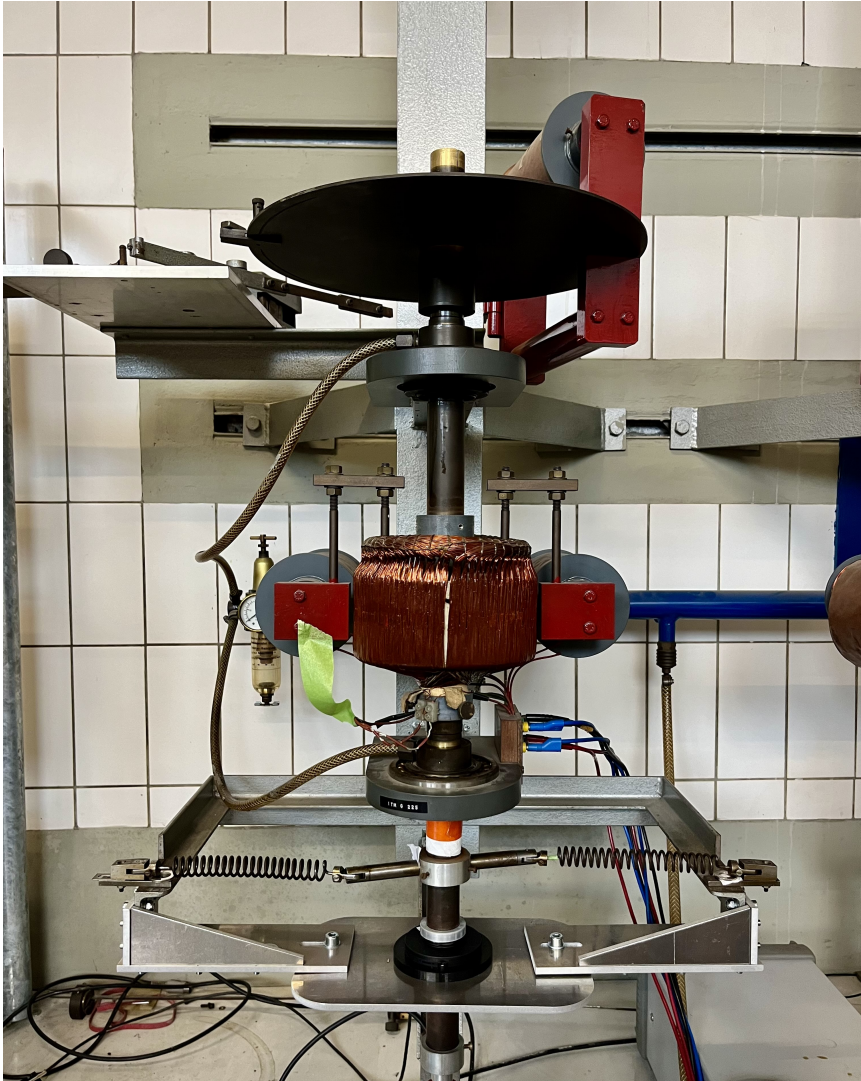
Figure 4.11: Experimental setup of a double-well oscillator created by the geometrical nonlinearities of coil springs
