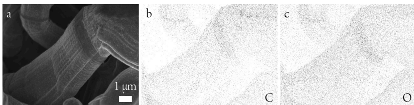
Figure 6.5: Investigation of the chemical composition by EDX. (a) SEM image, (b) map of the carbon distribution, and (c) map of the oxygen distribution. Reprinted from Becherer et al. [177]
