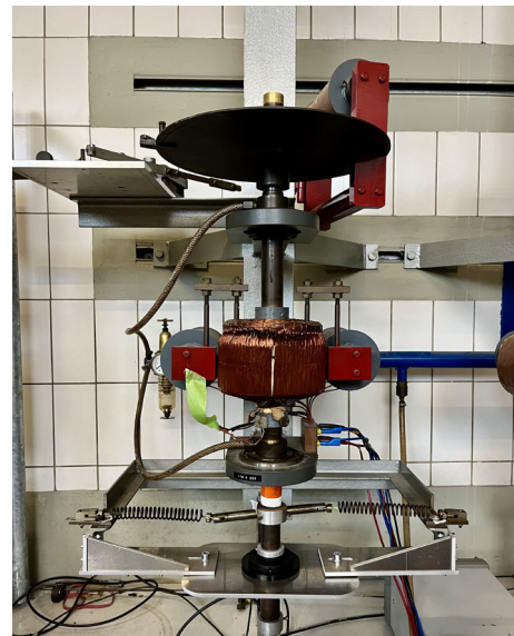
Fig. 3 Experimental setup of a double-well oscillator created by the geometrical nonlinearities of coil springs
