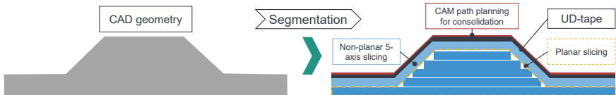
Figure 5-22: Four different segment types visualized using the example of a generic component to be manufactured from scratch
