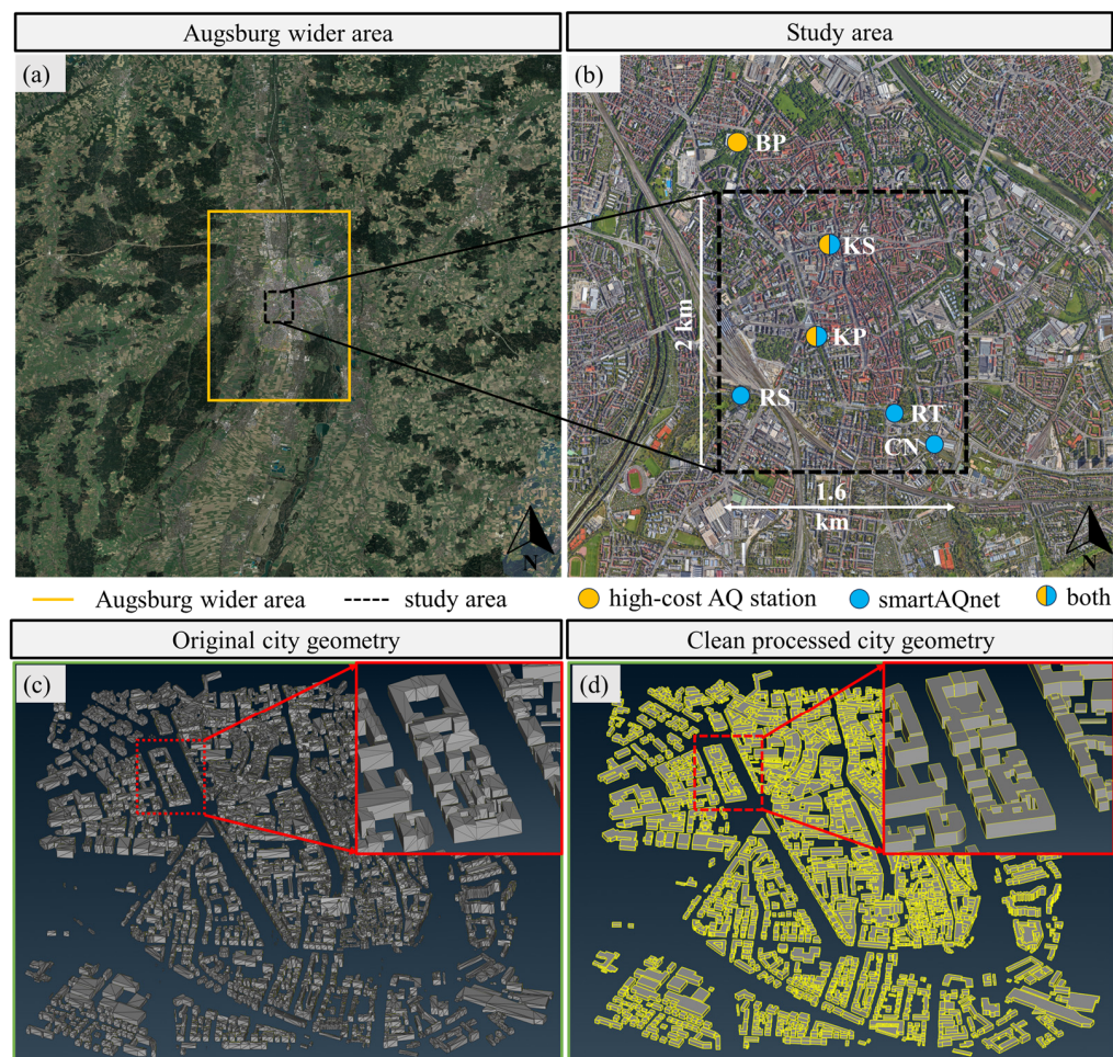
Figure 1. Wider area of interest (a). Test case area containing smartAQnet sensors and official AQ stations (b). OpenStreetMap (OSM) representation of the city (c) and clean geometry of the urban area used for CFD modeling (d).
