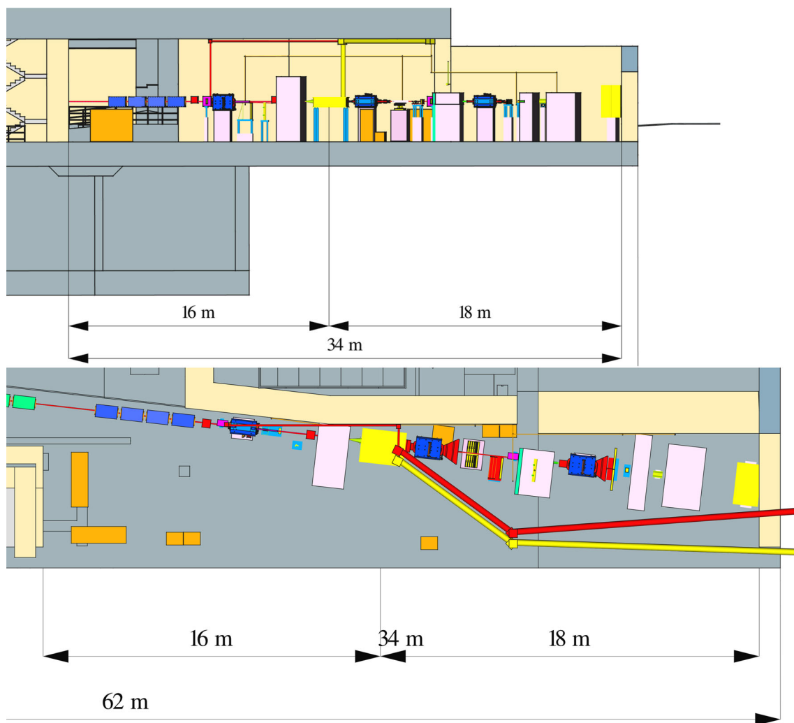
Fig. 254 CAD drawing of the LUXE area in UG03 of the XS1 access shaft building: (top) sideview and (bottom) topview. The building is shown in beige and grey, while the different experimental elements are shown in colours
