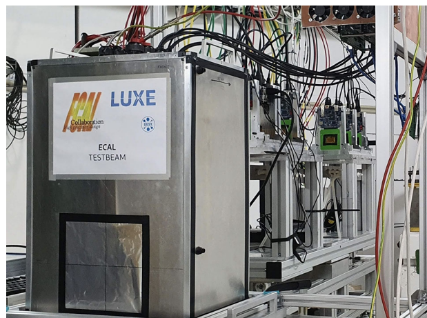
Fig. 106 The test-beam set-up for the measurements of the sensor response. Left in the foreground is the detector box with the sensors and FE-electronics inside. In the background on the right is the pixel telescope, used to measure the electron trajectory
