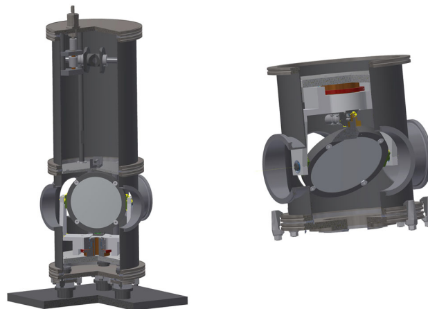
Fig. 35 Mirror mount design for the beamline for single circular beam for a (left) removable mirror and (right) standard mirror
