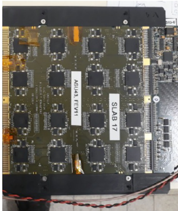
Fig. 104 A fully instrumented sensor plane for ECAL-E. The SKIROC2a ASICs are positioned on the sensor plane pad sensor
