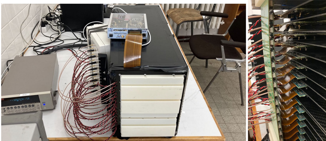
Fig. 91 Left: picture of the 15 layer stack of ECAL-E. Visible are the mechanical housing the HV and LV cabling and the flat Kapton cable for the readout of the 15,360 pads of the stack. Right: Zoom into the extremities of the stack to appreciate the compactness of the ensemble
