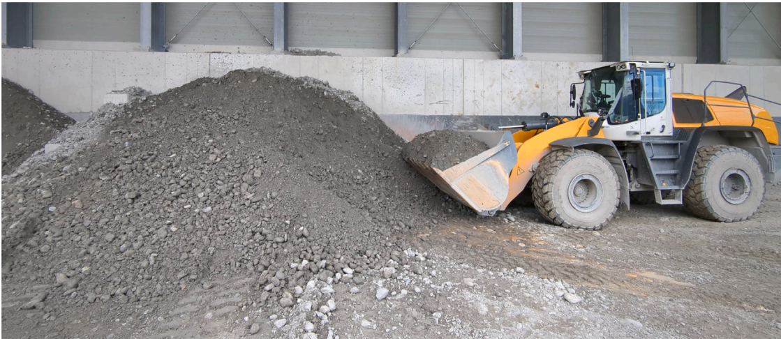
Fig. 10. Wheel loader and pile used for testing the neural network controller.
