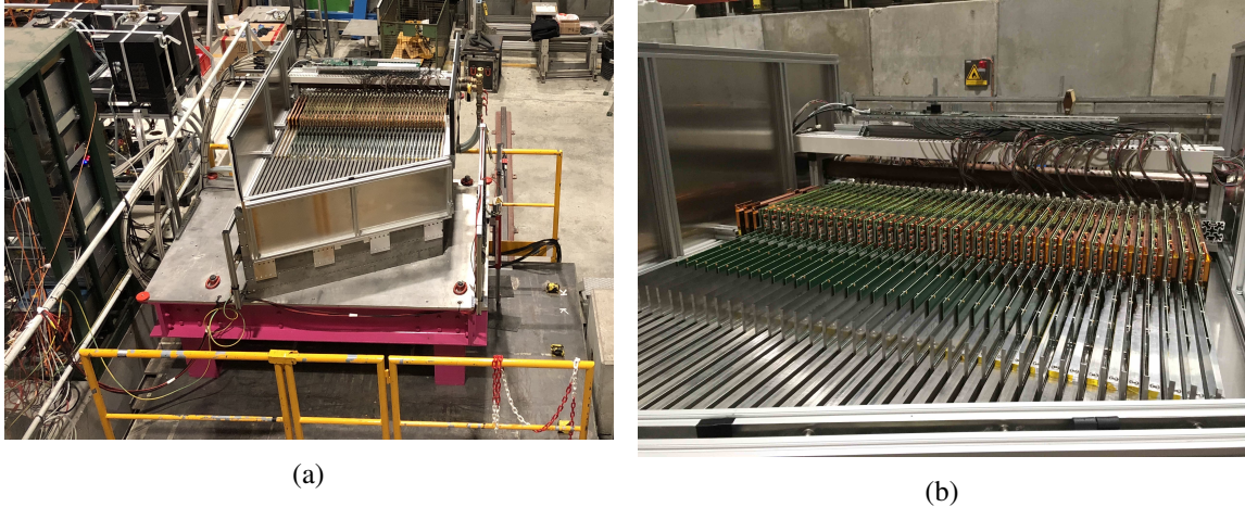
Figure 12. Photos of the assembled prototype: (a) Overview of the setup on the x-y-table in the H2 beam line at the CERN Super Proton Synchrotron. (b) Close-up of the interface boards sticking out of the absorber.
