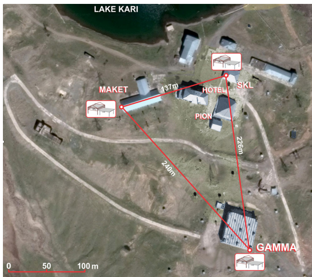
FIG. 1. STAND1 particle detector network at Aragats research station, 3200 m above sea level.
