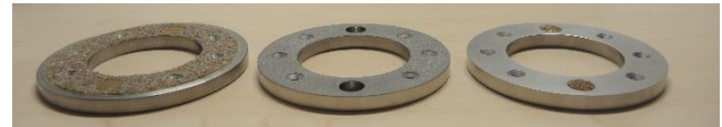
Figure 2. Different rough contact plates: with glued sand (left), coarse sandblasted (center), fine sand blasted (right).
