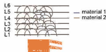
Fig. 10 Mismatch of layer height in multi-material printing leads to tilted columns or walls
