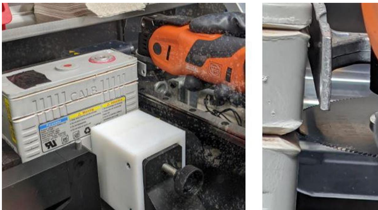
Figure 6: The cutting of Calb cell housing inside glovebox with oscillating cutting tool (left). The detail of the cutting profile (right) [107].
