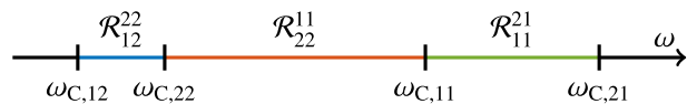
FIG. 5. Sketch of the ideal constraints of the characteristic frequency with the frequency axis \omega divided into the optimal intervals \mathcal{R}_i^j = [\omega_{C,i}, \omega_{C,j}] to tune the characteristic frequency for all tuples of group indices (i, j) \in \{(12, 22), (22, 11), (11, 21)\} . Herein, \omega_{C,i} denotes a characteristic frequency of one MEMS sensor.
