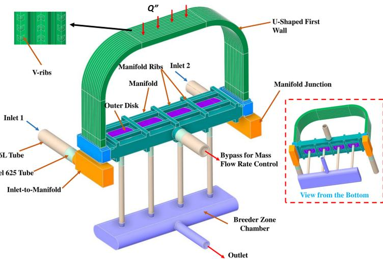
Fig. 1: Component nomenclature of FW - PMU
