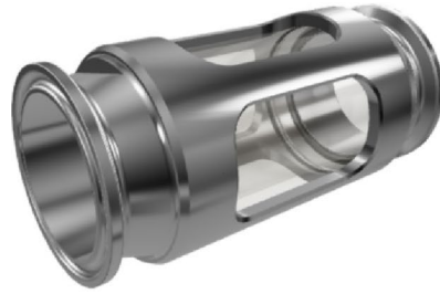
Fig. 3 Left: Sample holder for integration of catalyst samples into exhaust tailpipe. Right: Catalyst sample within sample holder
