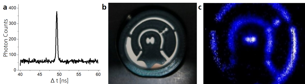
Figure 3.12: Results achieved with the proof-of-concept setup, shown in Figure 3.10. Two images are actually generated during measurement with this setup since the array consists of two sensor lines. However, only the image from the lower line is shown here. Further details on the measurement and image improvements can be found in the original publication [38]. (a) Coincidence evaluation of a line (line 26). The coincidence peak was reduced to 1 ns thanks to the corrections shown in Figure 3.11, and the CAR increased to about 4. (b) The transmission mask used for imaging, consisting of a "ghost." (c) Coincidence image after background subtraction and image enhancement, as described in [135]. Due to the coupling, part of the image was cut off (bottom left). The dark vertical stripes were caused by noisy pixels that were filtered during data acquisition.
