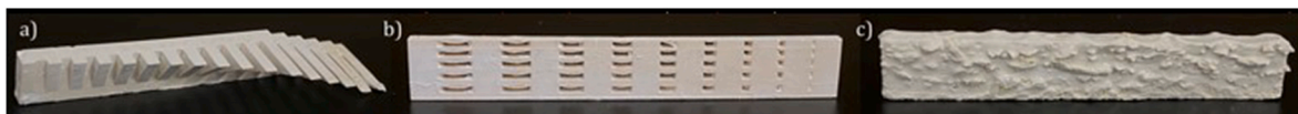
Fig. 5. Printed \text{ZrO}_2 parts: a) and b) with a curing energy of 105 \text{ mJ/cm}^2 leading to a high printing resolution and c) with an energy of 150 \text{ mJ/cm}^2 leading to a massive overpolymerization.
