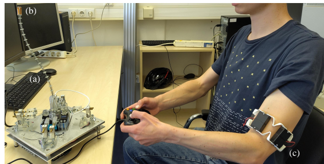
Fig. 1: A user controls the continuum robot (a) utilizing its capacitive proximity sensor (b) positioned at the TCP, while receiving vibrational feedback via the bracelet (c) placed on the upper arm.
