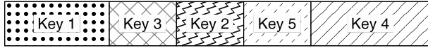
Figure 8: Keys generated to encrypt deltas modifying model parts for Figure 7. The OEM gets key 1 and 3; supplier 1 gets key 2, 3 and 5; supplier 2 3 gets keys 4 and 5
