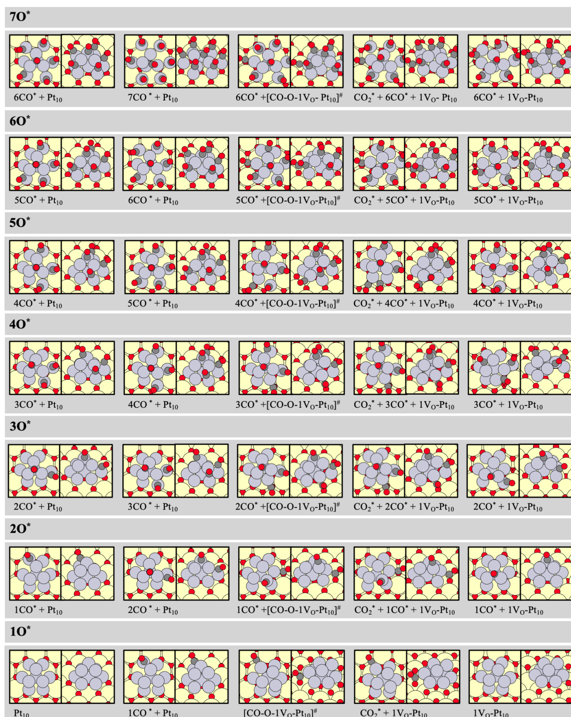
Figure 6.36.: Reaction mechanism of the CO oxidation on structure-optimized (1-7) CO^* + Pt_{10} clusters via the MvK mechanism adsorbed on a stoichiometric CeO_2(111) surface. Red circles represent O atoms, large yellow circles denote Ce atoms, dark gray circles represent C atoms, and light gray circles indicate Pt atoms. The total energies are listed in the Appendix in Table A.33.
