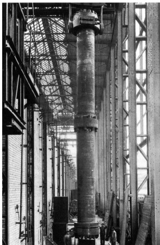
Figure 1.1.: High-pressure reaction furnace on an industrial scale around 1920. Reprinted with permission from 2 . ©2024 American Chemical Society.
