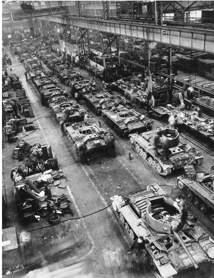
Figure 2: Valentine Tanks on the Assembly Line in the Tank Shop, Elswick Works, Newcastle upon Tyne, 28 September 1942 (TWAM ref. DX1529/1).
