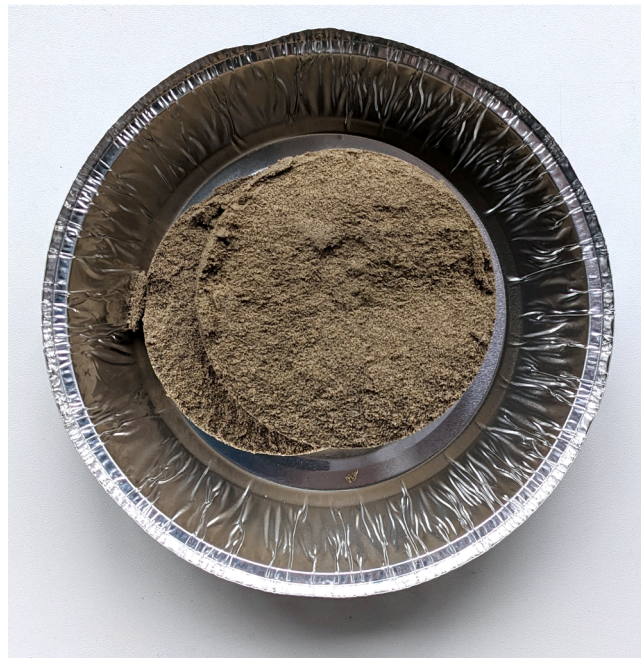
Fig. 9. Example of two 40 mm filter cakes: (a) 250 kPa filtration pressure, no air blow, average water content 20.2 w%, saturation 100 v%, average shear adhesion 0.9 \text{ kN m}^{-2} , average shear cohesion 1.2 \text{ kN m}^{-2} ; (b) 1250 kPa filtration pressure, 180 s air blow, 550 kPa air blow pressure, average water content 15.7 w%, average saturation 75 v%, average shear adhesion 3.1 \text{ kN m}^{-2} , average shear cohesion 5.0 \text{ kN m}^{-2} .
