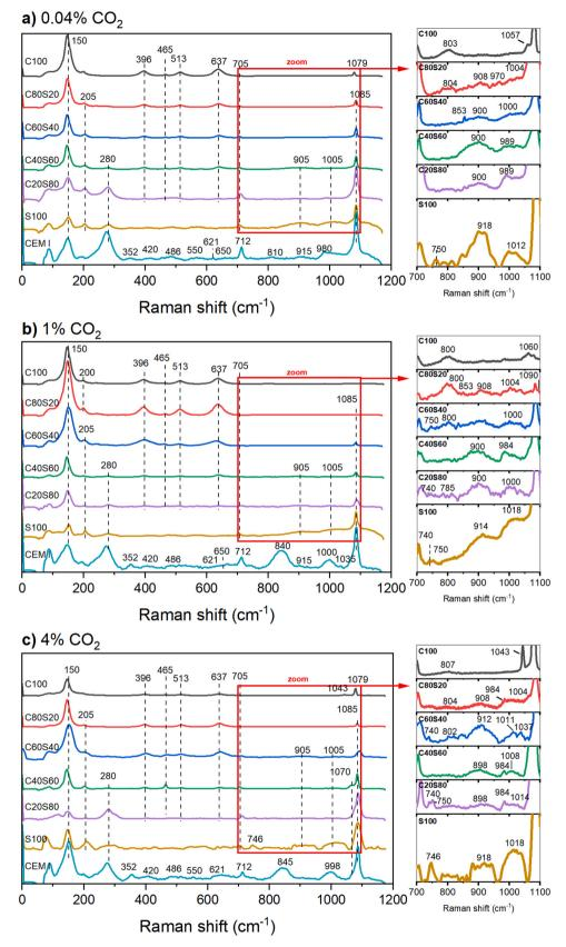
Fig. 5. Raman spectra of the pastes after a) 200 days of carbonation at natural  $CO_2$  concentration, b) 91 days of carbonation at 1 %  $CO_2$ , and c) 91 days of carbonation at 4 %  $CO_2$ .
