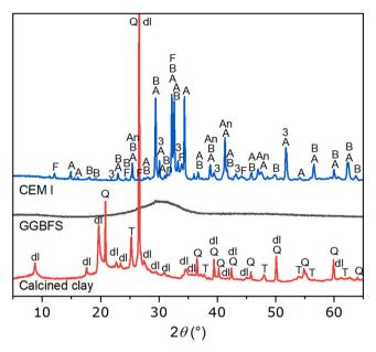
Fig. 1. XRD patterns of the solid binder starting materials. Major reflections are labelled 3: aluminate  $(C_3A)$ ; A: alite; An: anhydrite; B: belite; dI: dehydroxylated illite/muscovite; F: ferrite  $(C_4AF)$ ; Q: quartz; T: anatase.
