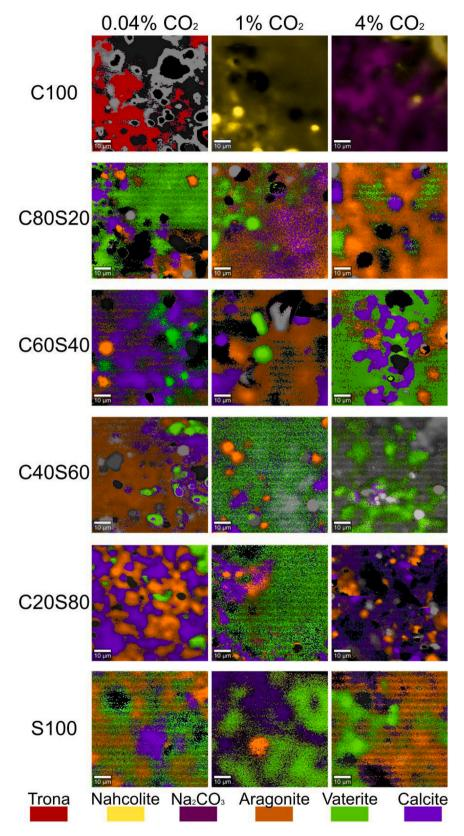
Fig. 6. Raman phase maps of the alkali-activated pastes after 200 days of carbonation at natural  $CO_2$  concentration, 91 days of carbonation at 1 %  $CO_2$ , and 91 days of carbonation at 4 %  $CO_2$ .
