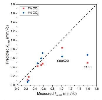
Fig. 9. Coefficients of carbonation at natural  ${\rm CO_2}$  concentration, predicted from the measurements under accelerated conditions and application of Eq. (1), versus measured coefficients of carbonation at natural  ${\rm CO_2}$  concentration. The dashed line is the line of equality.
