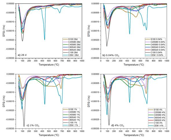
Fig. 4. DTG curves of the pastes after a) 28 days of curing, b) 200 days of carbonation at natural CO<sub>2</sub> concentration, c) 91 days of carbonation at 1 % CO<sub>2</sub>, and d) 91 days of carbonation at 4 % CO<sub>2</sub>.
