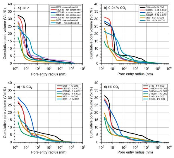
**Fig. 7.** Cumulative pore entry size distributions, determined by mercury intrusion porosimetry, of the pastes after a) 28 days of curing, b) 200 days of carbonation at natural CO<sub>2</sub> concentration, c) 91 days of carbonation at 1 % CO<sub>2</sub>, and d) 91 days of carbonation at 4 % CO<sub>2</sub>.
