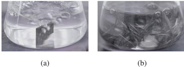
**Figure 3.9:** (a) Drop of a specimen in sulfuric acid in Erlenmeier flask and (b) dispersion of the detached fibers. Courtesy of FIBRE Bremen. Extracted from Blarr et al. [188].
