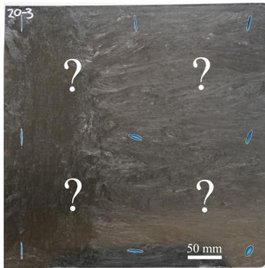
**Figure 2.11:** Visualization of the interpolation problem: Nine measured tensors of 10 mm × 10 mm × 3 mm specimens are shown as blue tensor glyphs at the corresponding extraction points. A transparent photo of an original plate with the dimensions 400 mm × 400 mm × 3 mm is shown in the background. The behavior of the fiber orientation between the small measured areas is unknown. Based on Blarr et al. [17].
