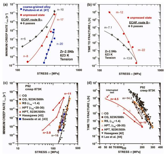
Fig. 35. Stress dependences of (a,c) the minimum creep rate  $\dot{\epsilon}_{min}$ , and (b,d) the time to fracture  $t_f$  for (a,b) Zr-2.5 Nb (wt%) alloy [754] and (c,d) P92 steel [756]. The creep results for coarse-grained materials published by Pahutova *et al.* [759], Hasegawa [760], Sawada *et al.* [761], and Lee *et al.* [762] are also listed.
