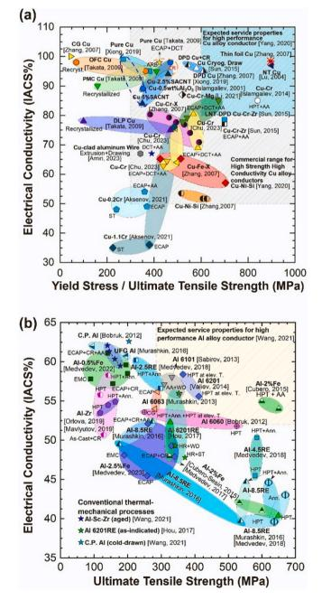
Fig. 40. Electrical conductivity with respect to strength in (a) copper and (b) aluminum alloys [834].
