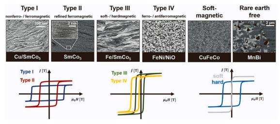
Fig. 43. Different types of microstructures which can be generated by HPT applied to powder/powder blends and their corresponding schematic magnetic hysteresis curves [841].
