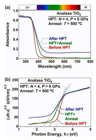
Fig. 44. (a) UV-Vis absorbance spectra and (b) bandgap calculation by the Kubelka-Munk theory for  $TiO_2$  before and after HPT processing and after HPT followed by annealing [639].
