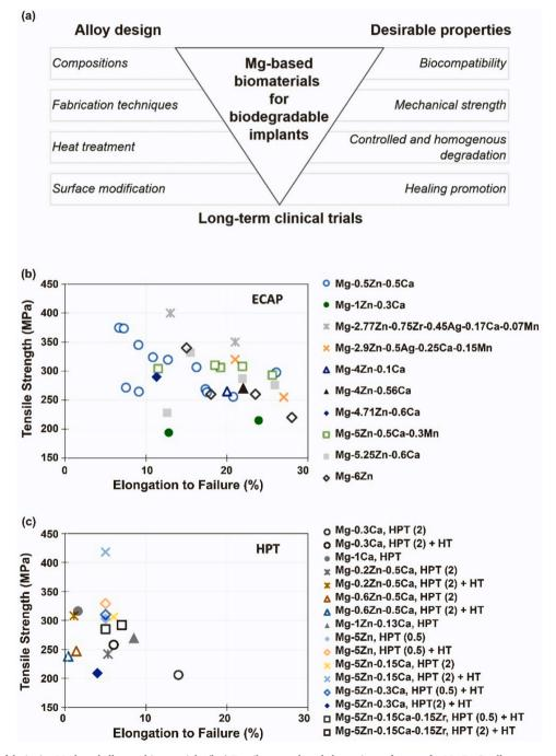
Fig. 62. (a) Concept of designing Mg-based alloys as biomaterials. (b,c) Tensile strength and elongation at fracture for Mg-Zn-Ca alloys processed by (b) ECAP and (c) HPT (the numbers in parentheses for HPT-processed samples indicate the number of rotations and 'HT' indicates a subsequent heat treatment) [1389].
