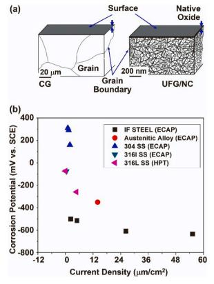
**Fig. 60.** (a) Differences between coarse grain (CG) and ultrafine/nanograined (UFG/NC) in the formation of native oxide passivation layer in steels [1276]. (b) Comparison of corrosion potential and current density between different steels processed by SPD: IF steel by ECAP [1295], austenitic steel by ECAP [1296], 304 stainless steel by ECAP [1297], 316 L stainless steel by ECAP [1276, 1298] and 316 L stainless steel by HPT [1299, 1300].
