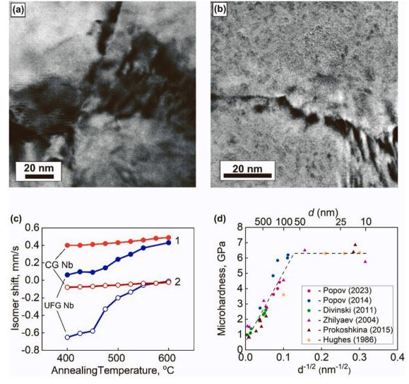
**Fig. 19.** (a,b) Stepwise boundaries in HPT-processed (a) niobium and (b) nickel [407]. (c) Isomer shifts of <sup>57</sup>Co(<sup>57</sup>Fe) spectral lines versus annealing temperature in coarse-grained niobium (red lines and symbols) and UFG niobium (blue lines and symbols) [406]. (d) Microhardness versus grain size (d) in nickel processed by various techniques [407].
