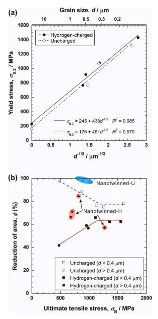
**Fig. 58.** (a) Grain size dependence of yield stress and (b) relationship between area reduction and ultimate tensile strength for 304 stainless steels with different grain sizes [848].
