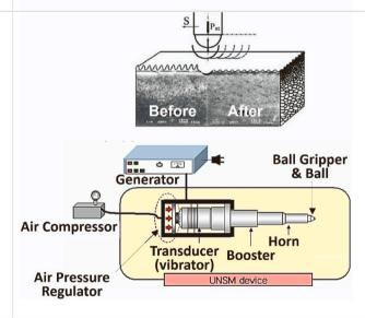
Rotating pins ultrasonic peening (RPUP) [131]
