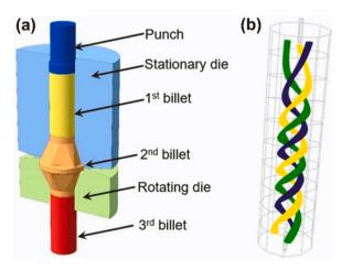
**Fig. 6.** (a) Schematics of the HPTE process with three billets inside the die [184]. (b) X-ray tomography reconstruction of aluminum wires embedded into the copper billet after HPTE processing with translational velocity  $\nu = 6$  mm/min and rotational velocity  $\omega = 1$  rpm (aluminum wires are shown in three different colors for better visualization) [185].
