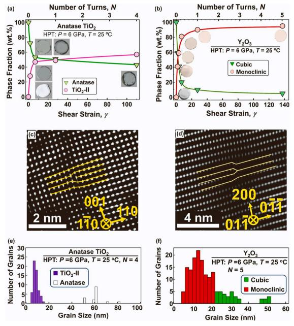
Fig. 27. (a,b) Influence of plastic shear strain on the fraction of high-pressure phases in (a) TiO<sub>2</sub> [582] and (b) Y<sub>2</sub>O<sub>3</sub> [583] after HPT processing. (c,d) Formation of dislocations during phase transformations of (c) ZrO<sub>2</sub> [584] and (d) TiO<sub>2</sub> [582] after HPT processing. (e,f) Grain size effect on the stability of high-pressure (e) TiO<sub>2</sub>-II [582] and (f) monoclinic Y<sub>2</sub>O<sub>3</sub> [583] after HPT processing.
