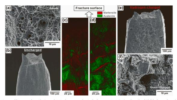
Fig. 57. SEM images of fracture surface, side view and EBSD phase maps at longitudinal cross-section in (a–c) uncharged and (d–f) hydrogen-charged specimens of ordinary-grained type 304 stainless steel [1237].
