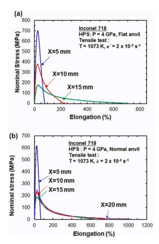
**Fig. 11.** Stress-strain curves of tensile specimens extracted from samples processed using (a) flat-type and (b) groove-type anvils of incremental-feeding HPS for sliding distances of 5, 10 and 15 mm (tensile tests were performed at 1073 K with an initial strain rate of  $2 \times 10^{-2}$  s<sup>-1</sup> [160].
