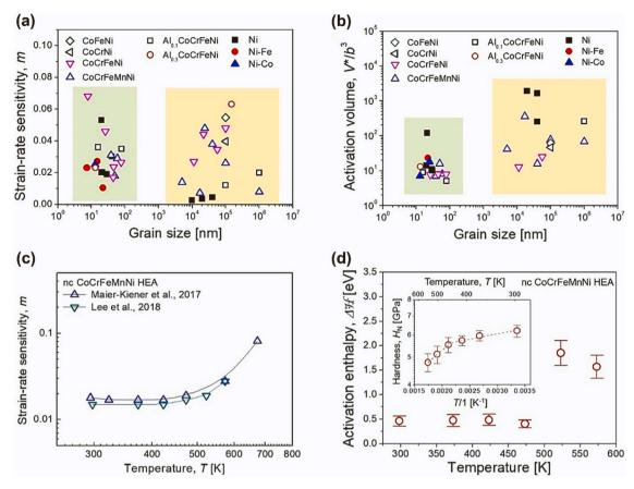
Fig. 80. Variations in (a) strain rate sensitivity and (b) activation volume of various FCC metals and alloys as a function of grain size [1671, 1674, 1685–1704]. (c,d) Results of high-temperature nanoindentation experiments for HPT-processed nanocrystalline CoCrFeMnNi HEA [505, 1690].
