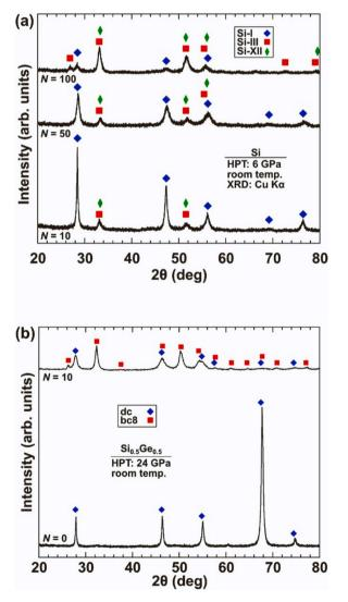
**Fig. 87.** XRD profiles of (a) silicon processed by HPT for different rotations (N) [1810] and (b) Si<sub>0.5</sub>Ge<sub>0.5</sub> processed by pure compression (N = 0) and N = 10 turns of HPT [1812].
