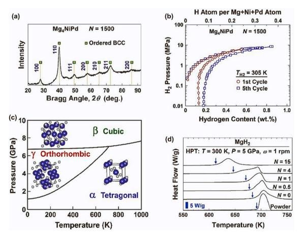
Fig. 53. (a) XRD pattern of Mg<sub>4</sub>NiPd after 1500 HPT turns [359]. (b) Pressure-composition isotherm of Mg<sub>4</sub>NiPd at 305 K [359]. (c) Pressure-temperature phase diagram of MgH<sub>2</sub> [515]. (d) Heat flow in differential scanning calorimetry for MgH<sub>2</sub> processed by HPT for various turns [515].
