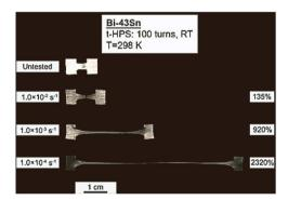
**Fig. 37.** Appearance of Bi-43Sn (wt%) samples after processing by t-HPS for 100 turns and pulling to failure at 298 K [224]: the elongation of 2320% exceeds the elongation of 1950% reported in early experiments by Pearson [24].
