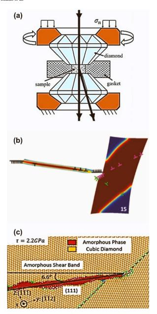
**Fig. 29.** (a) Schematic of RDAC. (b) Phase-field approach results showing dislocation pileup in the left grain produces a step at the grain boundary (superdislocation) with a strong stress concentrator leading to phase transformation and dislocation slip in the right grain [624]. (c) Molecular dynamics results showing dislocation pileup in the right grain produces a step at the grain boundary in Si-I phase and amorphization in the left grain [623].
