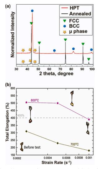
**Fig. 81.** (a) XRD patterns of  $Mo_{7.5}Fe_{55}Co_{18}Cr_{12.5}Ni_7$  HEA before (annealed) and after HPT processing [1650]. (b) Elongation versus strain rate plot for HPT-processed  $Mo_{7.5}Fe_{55}Co_{18}Cr_{12.5}Ni_7$  before and after tensile testing at elevated temperatures [1727].
