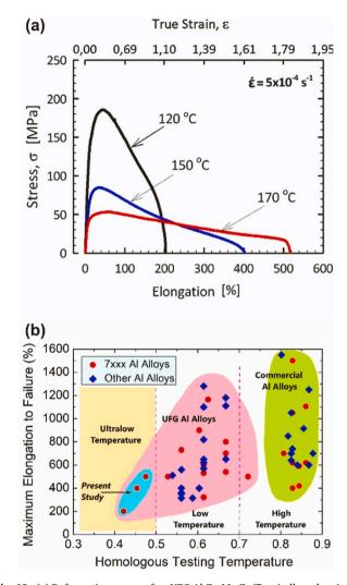
**Fig. 68.** (a) Deformation curves of an UFG Al-Zn-Mg-Zr (7xxx) alloy, showing a record total elongation higher than 500% at 443 K (homologous temperature: 0.47) [812]. (b) Significance of the UFG structure having grain boundaries segregated by solute atoms, resulting in ultralow-temperature superplasticity in the Al-Zn-Mg-Zr alloy (denoted as Present Study) [812].
