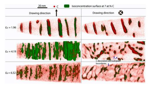
Fig. 72. Evolution from an initially lamellar structure (strain:  $\varepsilon_d = 1.96$ ) to a ferritic subgrain structure with carbon either supersaturated in the matrix or segregated to subgrain boundaries (strain:  $\varepsilon_d = 6.52$ ) by straining [682].
