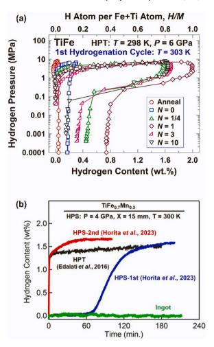
**Fig. 55.** (a) pressure-composition isotherms of TiFe at 303 K for annealed sample, sample processed by compression under 6 GPa (N=0) and samples processed by HPT for N=1/4–10 turns [1136]. (b) Variation of hydrogen content against hydrogenation time at room temperature after the first and second exposure to hydrogen under a pressure of 2 MPa for Ti-Fe-Mn intermetallic processed by HPS including as-received ingot and HPT-processed disc [1186].
