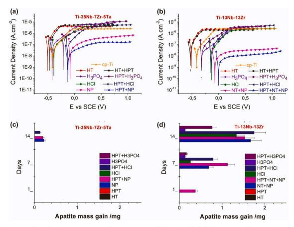
**Fig. 71.** (a,b) Corrosion behavior shown by potentiodynamic polarization curves recorded in simulated body fluid (SBF) at 310 K for (a) Ti-13-Nb-13Zr (TNZ) and (b) Ti-35 Nb-7Zr-5Ta (TNZT) alloys compared to commercially pure (CP) titanium with and without HPT processing. (c,d) Mass gain of apatite after immersing samples in SBF as a function of the soaking time, comparing treated and untreated surfaces of (c) TNZT and (d) TNZ before and after HPT processing [556, 1550, 1553, 1554, 1563].
