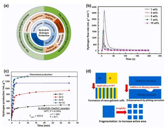
Fig. 50. (a) Materials used for hydrolytic hydrogen production [1038]. (b) Hydrolytic hydrogen flow rate curves of Al - 5 wt% LiH - x wt% Ga<sub>2</sub>O<sub>3</sub> (x = 1, 3, 5, 7 and 10) at 298 K [1039]. (c) Hydrolytic hydrogen production curves of HPT-processed Al-30Bi-10 C (wt%) composite with different HPT turns [1040]. (d) Combination of three strategies to promote aluminum hydrolysis by high-pressure torsion [1040].
