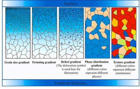
Fig. 95. Micro-schematic diagram of various gradient structures [1955].
