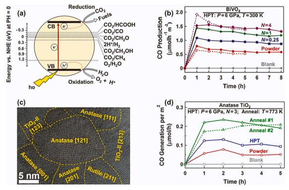
**Fig. 46.** (a) Schematic of photocatalytic CO<sub>2</sub> conversion mechanism [981]. (b) Photocatalytic CO production rate of BiVO<sub>4</sub> versus time for powder and samples processed by HPT with 0.25, 1 and 4 turns [961]. (c) High-resolution TEM image of sample processed by HPT containing TiO<sub>2</sub>-II high-pressure phase [985]. (d) Rate of CO generation for TiO<sub>2</sub> samples before HPT, after HPT and after HPT and annealing [985].
