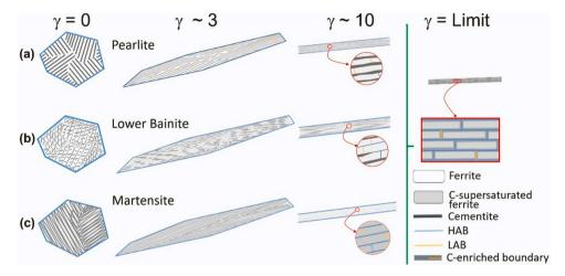
Fig. 73. Schematic illustration of the structural evolution of (a) pearlitic, (b) bainitic and (c) martensitic structures during quasi-constrained HPT deformed up to current technological limits [1583].
