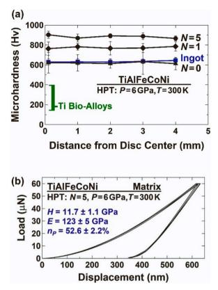
**Fig. 63.** (a) Variation of Vickers microhardness against distance from disc center for ingot and sample processed by HPT. For comparison, hardness for TiAlFeCoNi after compression (N=0) and N=1 turn of HPT, as well as the hardness range for Ti-based biomaterials, were included. (b) Nanoindentation load against displacement for HPT-processed TiAlFeCoNi sample [1356].
