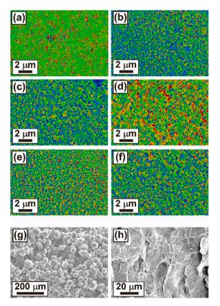
**Fig. 90.** (a-f): SEM micrographs of nanocomposites of LLDPE polymer with (a-c) 10 wt% of carbon nanotubes and (d-f) 20 wt% of carbon nanotube addition, after true strains of (a,d) e=0, (b,e) e=4.4, (c,f) e=8.5 [1861]. (g,h) Morphologies of compacted polypropylene powders after strains of (g) e=0 and (h) e=8.5 [1841].
