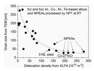
**Fig. 77.** The grain size versus the dislocation density obtained for FCC and BCC Al-, Cu-, Ni- and Fe-based conventional alloys and multi-principal element alloys (MPEAs) processed by HPT at room temperature [1667].
