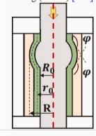
$\frac{\overline{\varepsilon}_{RPTS}}{=\frac{4}{\sqrt{3}}N\left[\cot\frac{\varphi}{2}\right]} + ln\frac{R_0 + R}{R_0 + r_0}$
