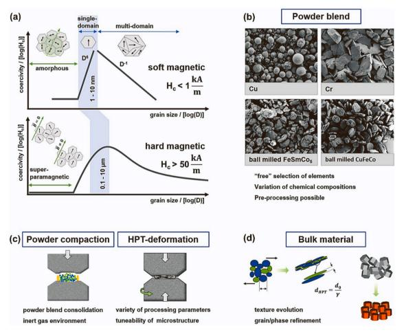
Fig. 42. (a) Schematic representation of coercivity ( $H_c$ ) as a function of grain size (D) for soft (upper graph) and hard magnetic (lower graph) materials (different logarithmic scales for  $H_c$  of soft and hard magnetic are used) [888–893]. (b) Powder blends for the HPT process, (c) schematic representation of powder-based HPT processes and (d) schematics of bulk materials produced by HPT from powder blends with enhanced microstructural features [841].
