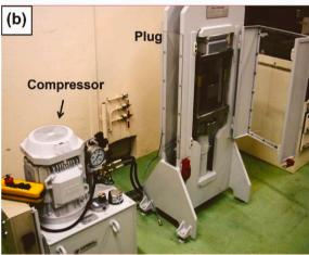
**Fig. 56.** (a) Fast Forging instrument of the drop type (sample is placed in an argon-filled chamber and can be also heated using an induction coil). (b) ECAP instrument (die can be heated on demand by resistive inserts placed in the die. The deformation rate can be controlled in both instruments by computer-connected sensors [1100].
