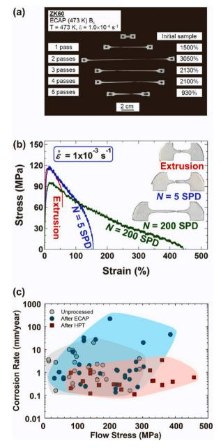
**Fig. 66.** (a) Appearance of tensile specimens of a ZK60 alloy processed by different number of passes of ECAP and tested at 473 K [1475]. (b) Stress vs. strain curves and appearance of tensile specimens of an Mg-8Li (wt%) alloy processed by extrusion and different number of turns of HPT and tested at room temperature [350]. (c) The corrosion rate of magnesium and magnesium alloys plotted as a function of the flow stress [1478].
