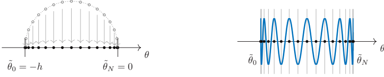
(a) Geometric intuition of the cosine in (3.2): the non-equidistant (one-dimensional) grid as a projection of equidistant circle points.
