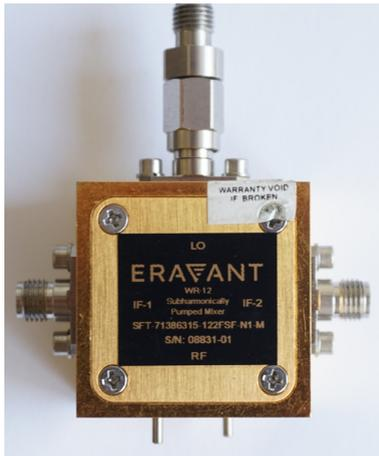
Fig. A.1: The subharmonic mixer employed in the measurement campaign.
