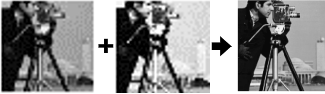
Figure 7.1: The process of combining two or more low-resolution or noisy images to form an high-resolution image of the underlying scene is called super-resolution. Figure adapted from [143].
