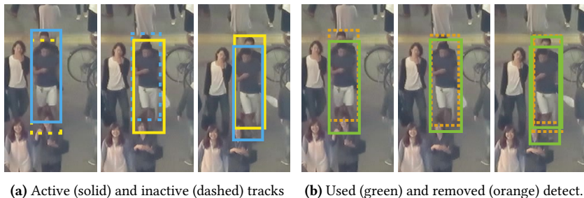
Figure 6.2: Failure of standard association (a) and available detections (b) under person-person occlusion. The removal of detections in the NMS is caused by too large overlaps.
