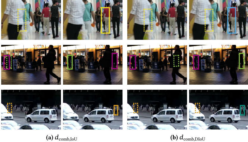
Figure 6.13: Qualitative comparison of using d_{\text{comb,IoU}} and d_{\text{comb,DIoU}} as association distance on example sequences from the MOT17, PP22, and SOMPT22 dataset (top to bottom). The DIoU prevents infeasible assignments with large spatial distances on the image (b), which cannot be done by the IoU within the combined distance measure, as the IoU is always zero for non-overlapping boxes, independent from their distance (a).
