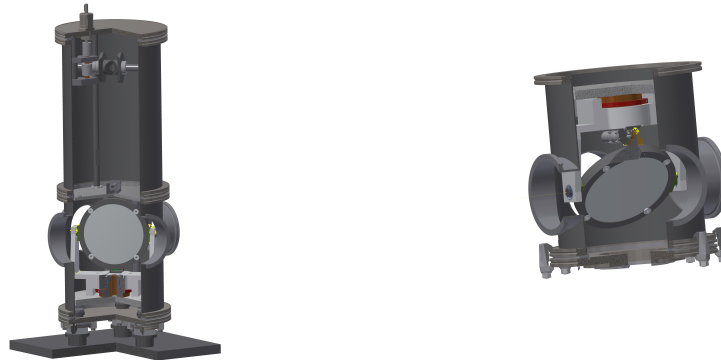
Figure 3.12: Mirror mount design for the beamline for single circular beam for a (left) removable mirror and (right) standard mirror.
