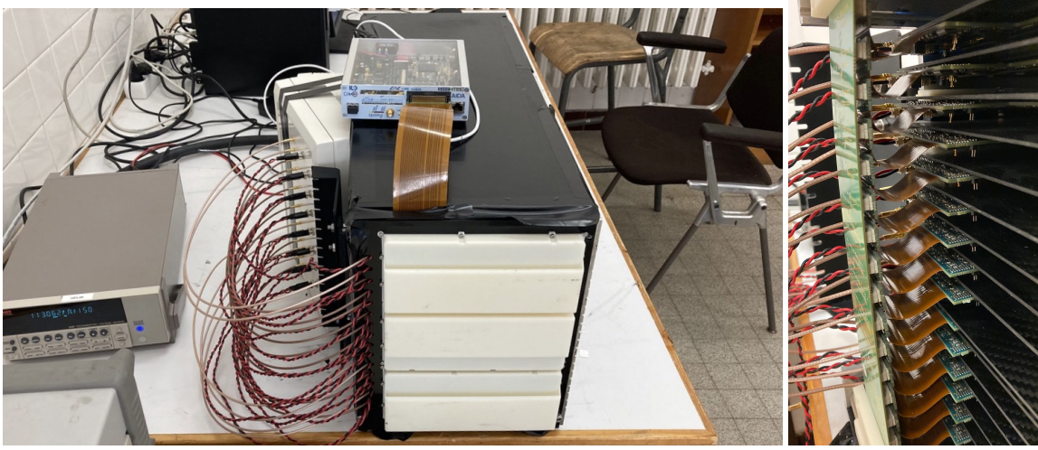
Figure 5.5: Left: picture of the 15 layer stack of ECAL-E. Visible are the mechanical housing the HV and LV cabling and the flat Kapton cable for the readout of the 15360 pads of the stack. Right: Zoom into the extremities of the stack to appreciate the compactness of the ensemble.
