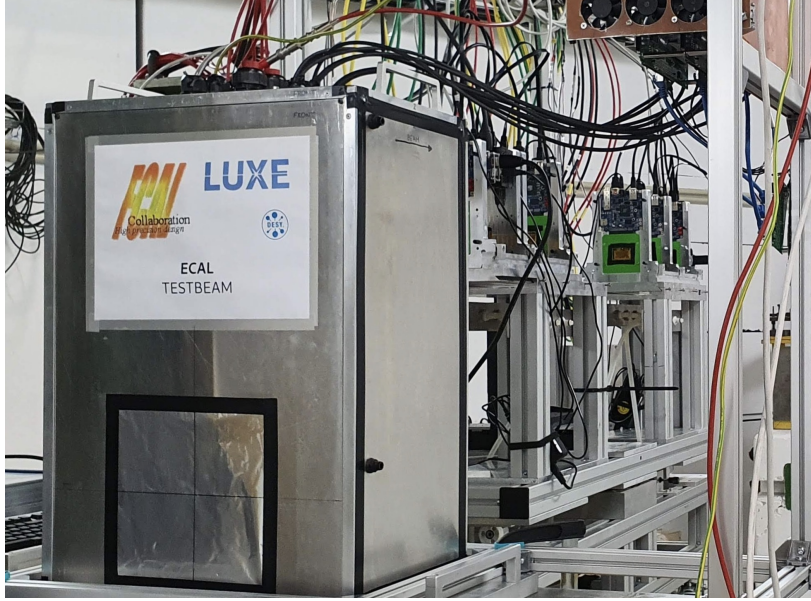
Figure 5.20: The test-beam set-up for the measurements of the sensor response. Left in the foreground is the detector box with the sensors and FE-electronics inside. In the background on the right is the pixel telescope, used to measure the electron trajectory.
