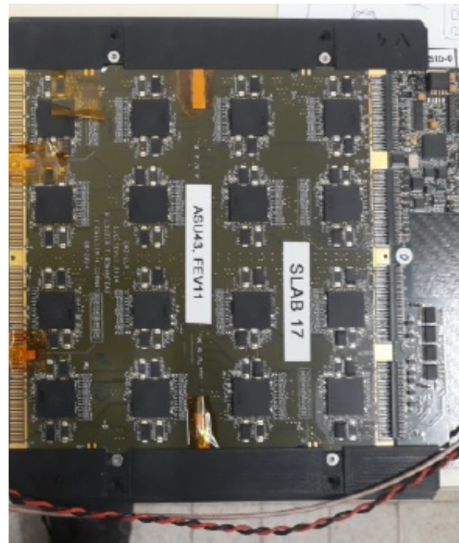
Figure 5.18: A fully instrumented sensor plane for ECAL-E. The SKIROC2a ASICs are positioned on the sensor plane pad sensor
