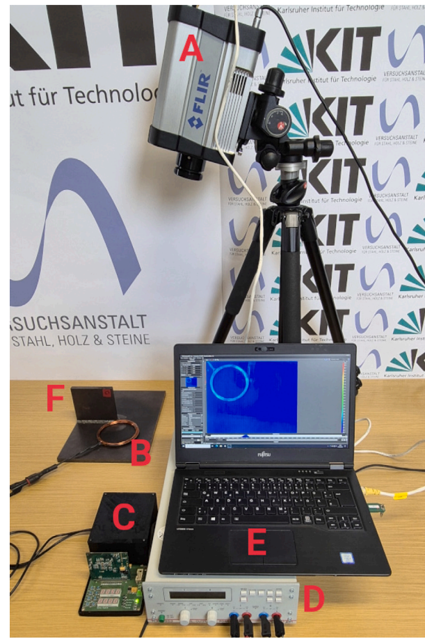
Fig. 2. Real time crack detection system. A: IR camera, B: coil, C: S2S unit, D: voltage supply, E: PC and F: steel specimen.
