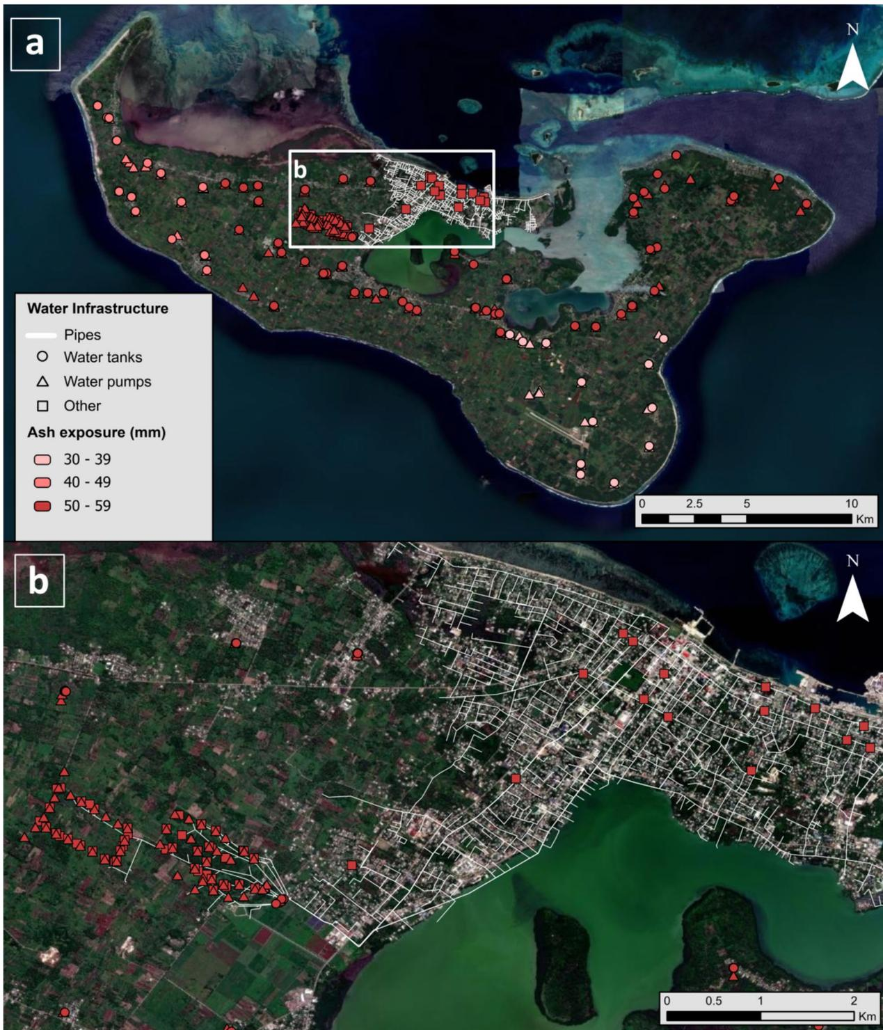
**Fig. 7** Water sector exposure. Source hazard data: USGS Ash3D; 30 km column height; 1-h duration; 0.5 km<sup>3</sup> (with umbrella), Source asset data: ADB 2021 database (The World Bank 2021). a The results
