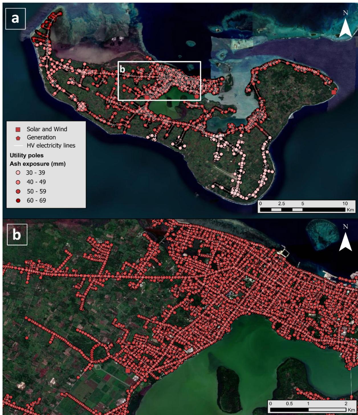
**Fig. 8** Electricity sector exposure. Source hazard data: USGS Ash3D; 30 km column height; 1-h duration; 0.5 km<sup>3</sup> (with umbrella), Source asset data: ADB 2021 database (The World Bank 2021). a The results
