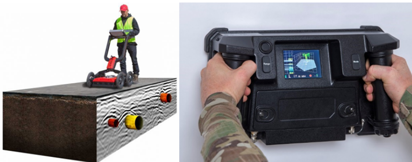
Fig. 1.2: (Left) A GPR system for mapping the location of the underground abandoned pipe, (right) a TWRI system that provides a clear position of people behind the wall.
