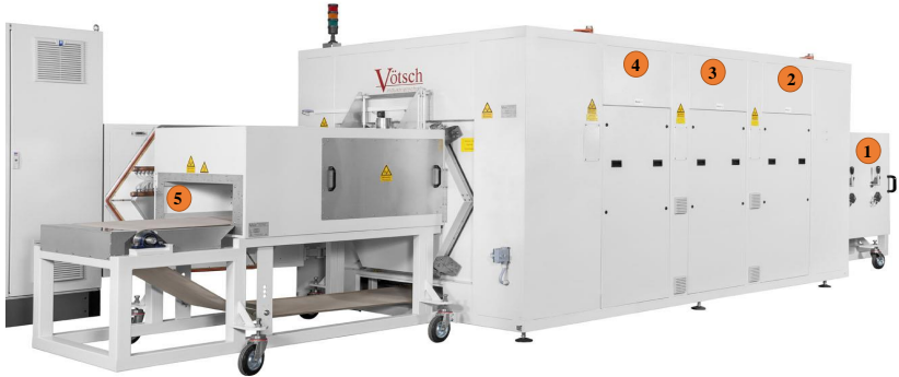
Fig. 1.4: A side view of the HEPHAISTOS microwave oven system. The main modules of the oven are represented by number tags 1, 2, 3, 4, 5. Tag 1 and Tag 5 represent the entrance of the wet foam and exit doors for the dry foam on the conveyor belt, respectively. Tags 2, 3, and 4 indicate the three modular heating systems which inbuilt the hexagonal cavity with high-power microwave heating sources and control system block.
