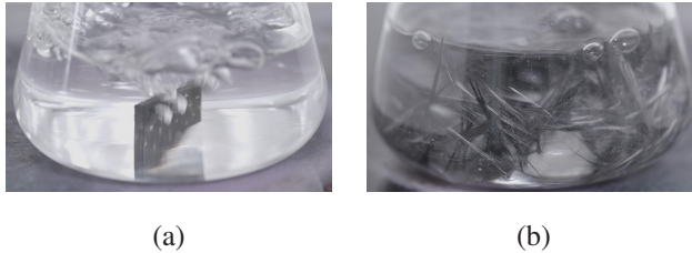
Figure 3.9: (a) Drop of a specimen in sulfuric acid in Erlenmeyer flask and (b) dispersion of the detached fibers. Courtesy of FIBRE Bremen. Extracted from Blarr et al. [188].
