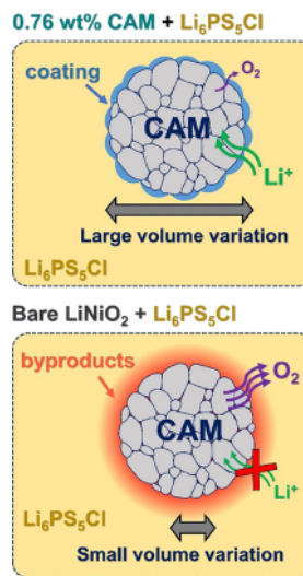
Figure 5. Schematic illustration of the working principle of the \text{LiNbO}_3 protective surface coating on the \text{LiNiO}_2 secondary particles.
