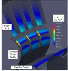
Example map of  $q_{||}$  calculated in SMITER for a 15MA Downward VDE [7], also [4]
