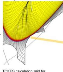
TOKES calculation grid for downward VDE CQ simulations
