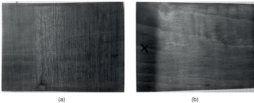
Figure 4.17: Specimens with (a) sanded and (b) sandblasted surface.
