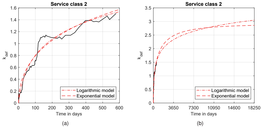
Figure 7.25: Creep factor k_{def} in SC2 for 600 days (a) and 50 years (b) with adjusted displacement data.
