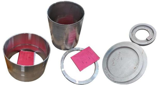
**Fig. 3.** Pre-machined stainless steel material for lower and middle assembly.
